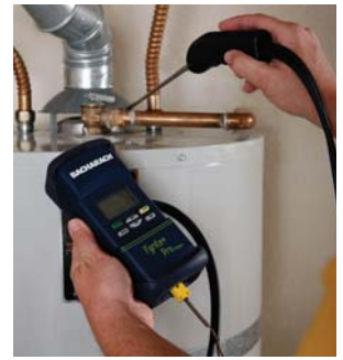
A Combustion Safety Test on your water heater will ensure that it is operating safely and efficiently.
